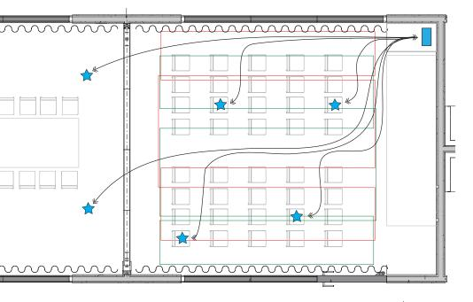
To ensure a loop system is Standard compliant the loop field has to be tested at multiple test points with a variety of signals and scenarios.
