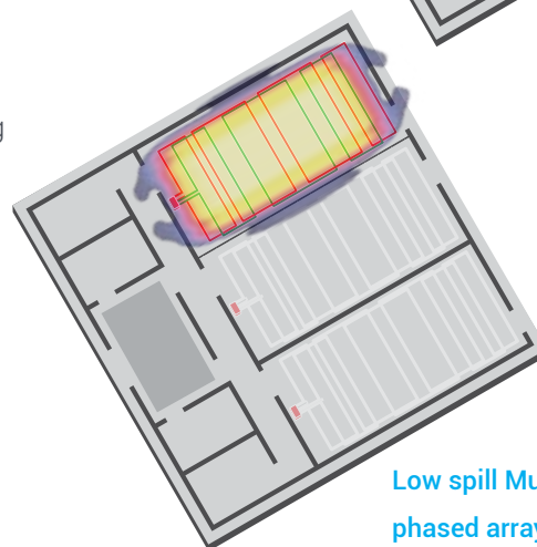
Standard perimeter loop (with overspill)
